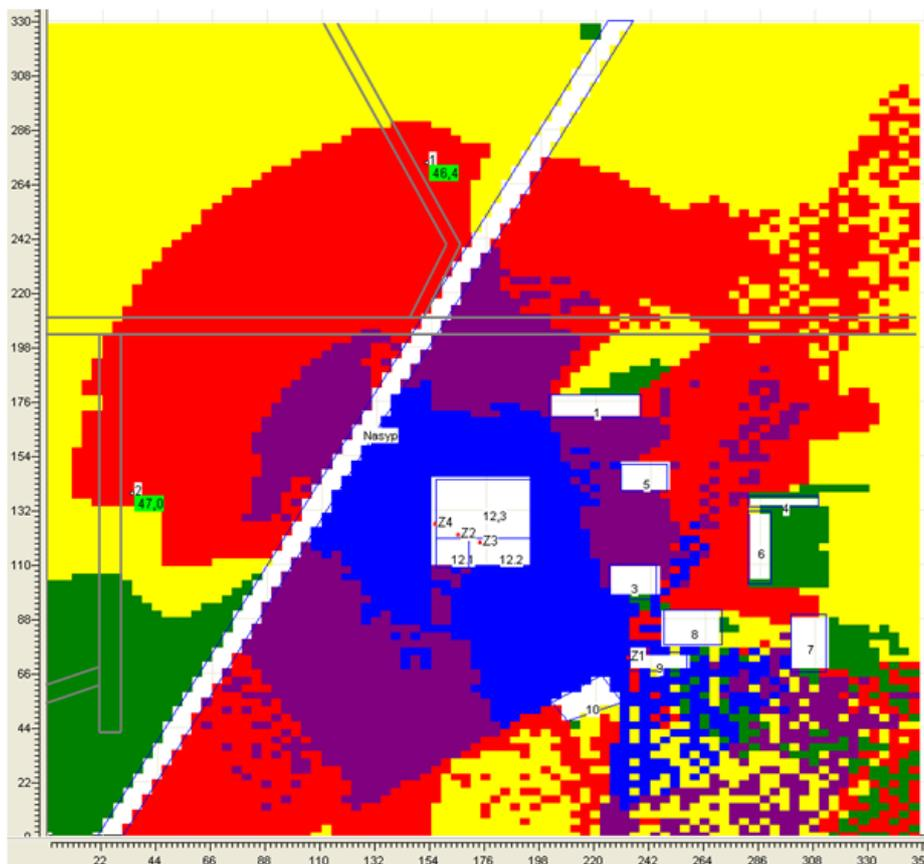
Figure 10. Acoustic map without noise sources reduction measures.
