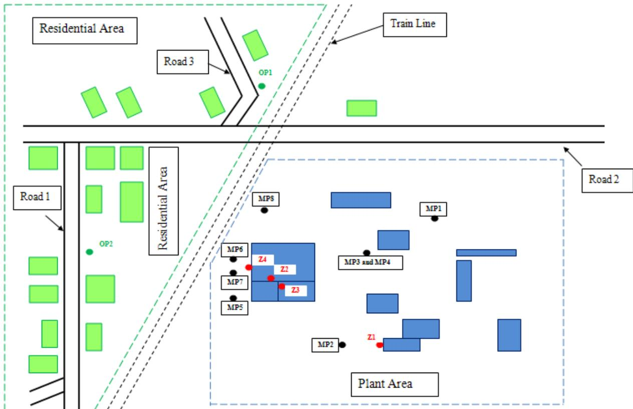
Fig. 9. Site map with measurement points and position of main noise sources.
