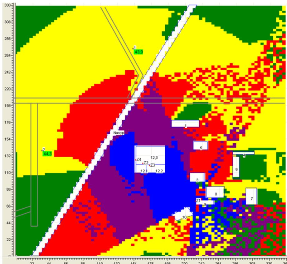
Fig.11. Acoustic map with assumed noise reduction for sources Z2, Z3 and Z4.
