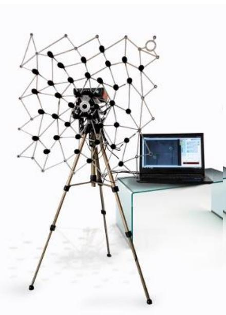
Fig.1. Acoustic camera CAE- Noise Inspector.
