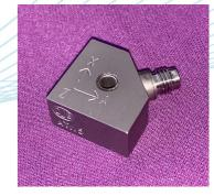
A lightweight general purpose triaxial vibration transducer comprising of three voltage output piezo-electric sensing elements mounted orthogonally within a titanium block with welded construction. The AT/15 is based upon the unique DJB Konic shear® design and offers a through hole mounting method which allows the user to orientate the connector and axes in the required direction for testing.
